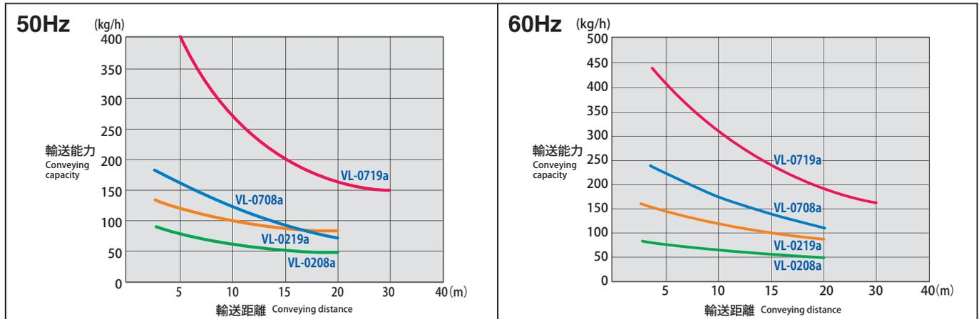
\* 輸送条件は見掛比重0.6ペレット \* Conveying capacity is under the condition that the bulk density of the pellet is 0.6.
