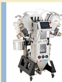
Gravimetric Batch Blender AUTOCOLOR II
