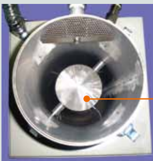
▲ 乾燥ホッパ(加熱・減圧) Drying hopper (heating / vacuum)
